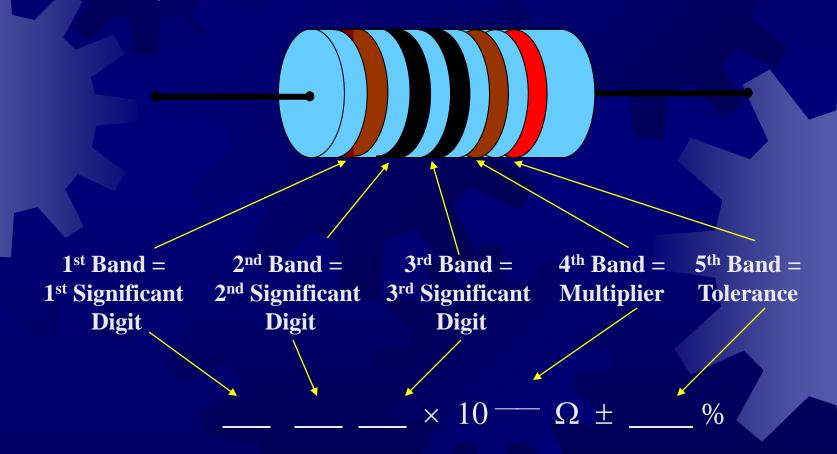
**Example 4.** Determine the nominal resistance and tolerance for the resistor shown below.
