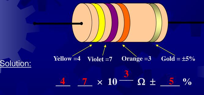
Resistor nominal value =  $47 \times 10^{3} \Omega$ =  $47,000 \Omega$ Tolerance =  $\pm 5\%$
